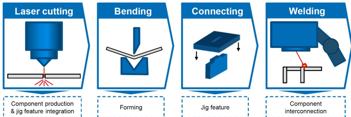
Example of a flexible process chain for the manufacture of body structures
